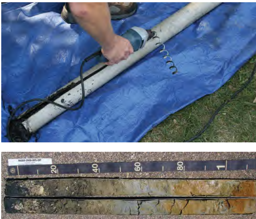
A core from subaqueous sampling. Top image—Cutting open the core with electric shears. Bottom image—A split core exposing the soil. One side is typically sampled, and the other may be stored and archived.
